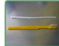
Pipe cleaner to clean the inside of the tube and toothbrush for outside
